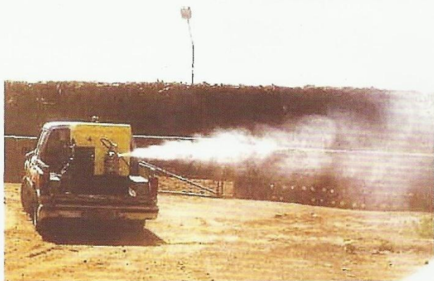
Cold Fogging/Aerosol Technique 20 - 200 Microns Droplet Size
